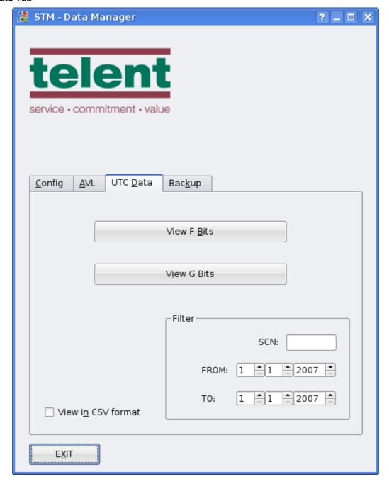
The UTC Data tab provides access to either F or G bits to/from the UTC system.
