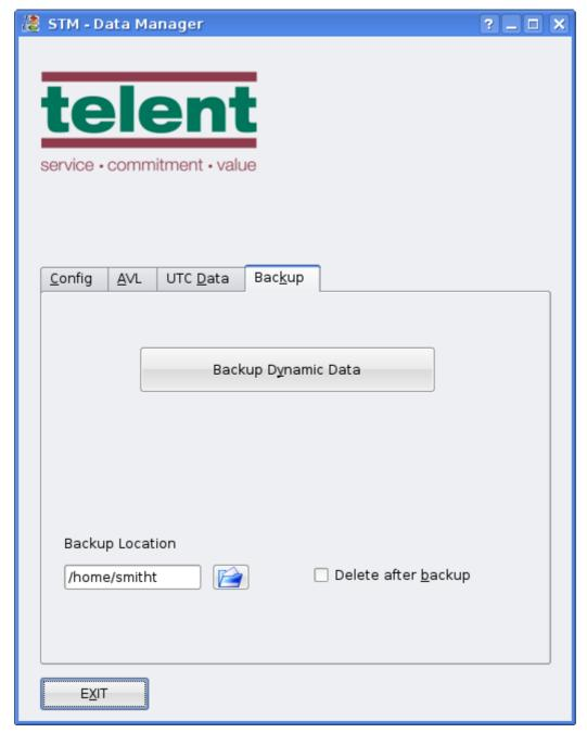
The Backup tab allows the user to backup the dynamic portions of the database for maintenance purposes.
